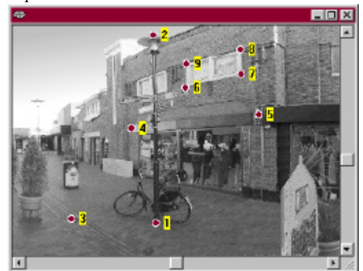
Using cycloramas you can quickly measure a lamppost (1,2), water drainage (3), overhead beam (4,5) and window frame (6-9)
